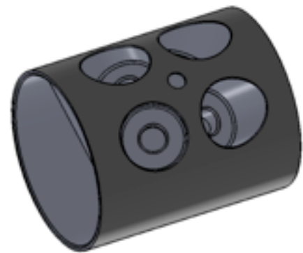
6 inch diameter AUV pressure hull with pockets for DVL piston transducers
