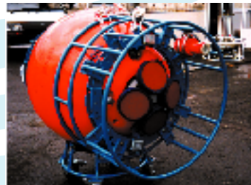
JAMSTEC uses LinkQuest acoustic modems to collect current data from moored ADCP periodically.
