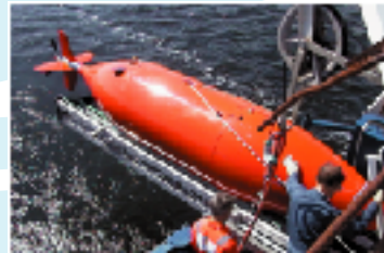
C&C Technologies uses LinkQuest acoustic modems to upload images from sidescan sonar and sub-bottom profiler on Hugin 3000 AUV
