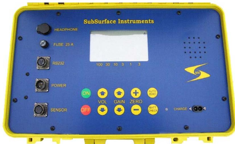
The LCD Bar graph fills to the left or the right side of the display depending on signal polarity. Left is Negative and right is Positive. As the signal increases in strength, the audio pitch increases in frequency.
