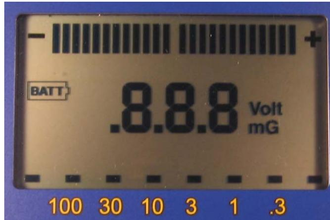
1. **Bar Graph (top)**.....Shows signal strength and polarity
